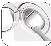
After every washing make sure that no foreign substance is left in the drum. If the holes on the bellow shown in the figure is blocked, open the holes using a toothpick.
